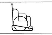
Ask the passenger to lean forward slightly and move the chair and handle forward until the Clamp Locks can be positioned under the curve in the handle.
