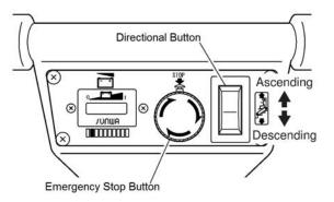
If it is necessary to use the Emergency Stop Button, ensure that Stair-Trac is examined by a qualified service person before it is used again.
