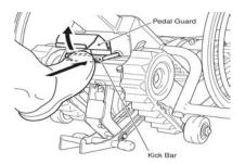
6. Raise the Support Handle and position the Holding Clamp Locks under the curves in the wheelchair handles.
