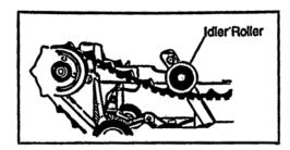
At a point halfway between the Idler Roller and the Drive Roller, press down firmly with your hand. At the closest point the track cogs should be 70mm  $\pm$  3mm (2 3/4 in  $\pm$  1/8 in) away from the flat part of the Drive Frame. You'll note that the tracks will touch the motor housing, but this is taken into consideration in the measurements. Check and adjust each track to obtain this measurement.
