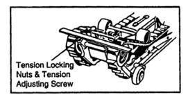
When decreasing tension, after turning the Adjusting Screw, press down on the tracks to remove any slack in them and to relocate the rear axle.
