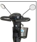
Removable mirror is adjustable and can be mounted on the left or right side of the control panel. Model no. ACC250
