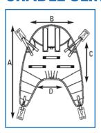
Designed for use with our new Jasmine lift. Comfort and support of the whole body and head are crucial for those with head, trunk and hip concerns. 4-point attachment clips onto the cradle bar for best positioning in horizontal-toseated or seated-to seated transfers. Head support is optional by removing rigidizers.
